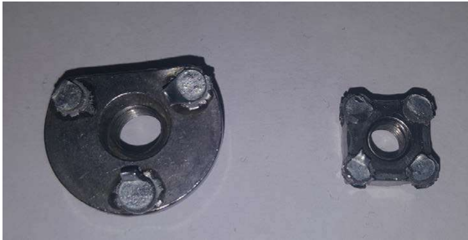
Figure 4. Nuts after the destructive test
