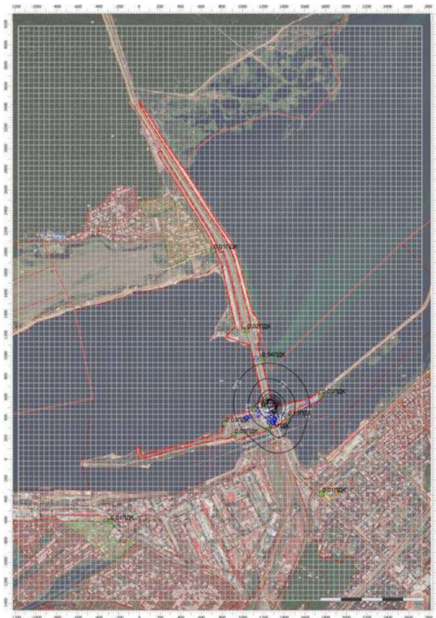
Figure 1. Isolines of dispersion of pollutants (industrial site No. 1 Main). Calculation code: 0616 (Dimethylbenzene (mixture of o-, m-, p-isomers) (Methyltoluene)). Parameter: Concentration of a harmful substance (in fractions of MPC)
