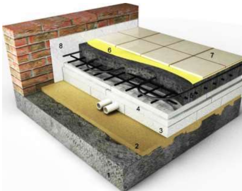
Figure 4. Insulation of a reinforced concrete slab above the basement
