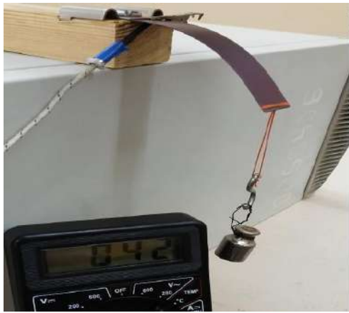
Figure 1. Plate deformation during cooling under load
