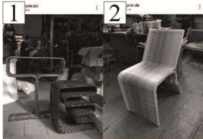
Figure 4. HDPE grinding caps and secondary polystyrene granules made from 3D printer printing: 1 – functional table with table chair; 2 – chair
