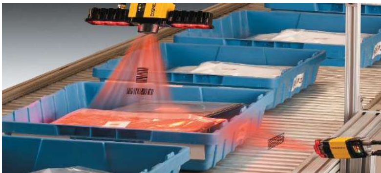
Figure. COGNEX Vision System for Product Quality Control [5].
